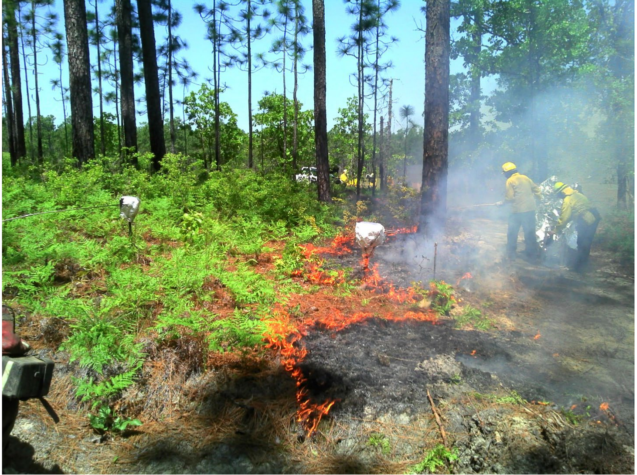
Figure 2 Fire behavior package 6 during burn 1. This package saw a peak total heat flux of 10.9\text{kW/m}^2 , peak air temperature of 423^\circ\text{C} , and registered a peak wind speed of 3\text{ m/s} .
