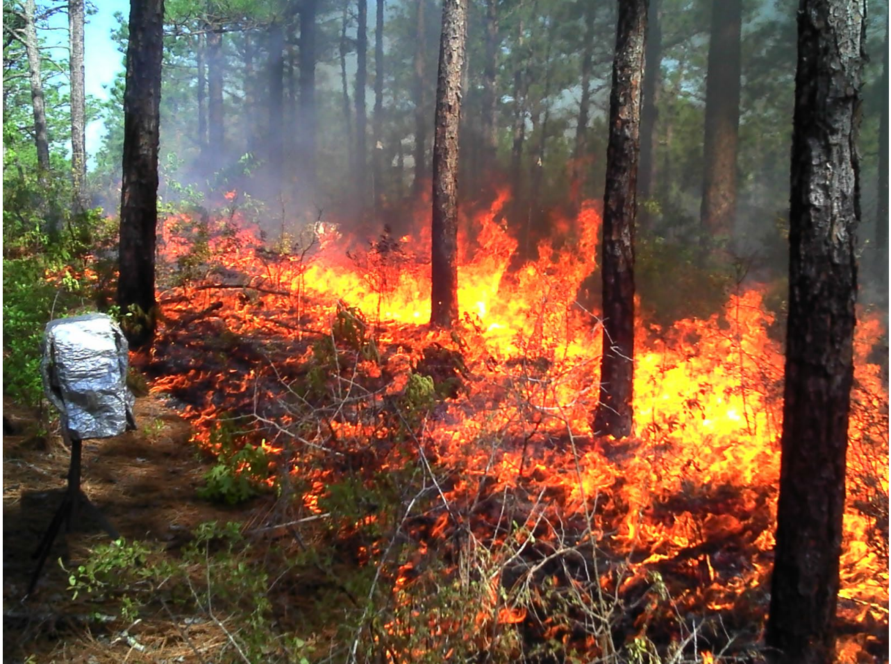
Figure 5 Fire behavior during burn 3 where a peak total heat flux value of 17.5\text{kW/m}^2 was registered along with a peak air temperature of 954^\circ\text{C} and peak wind speed of 4.5\text{m/s} .
