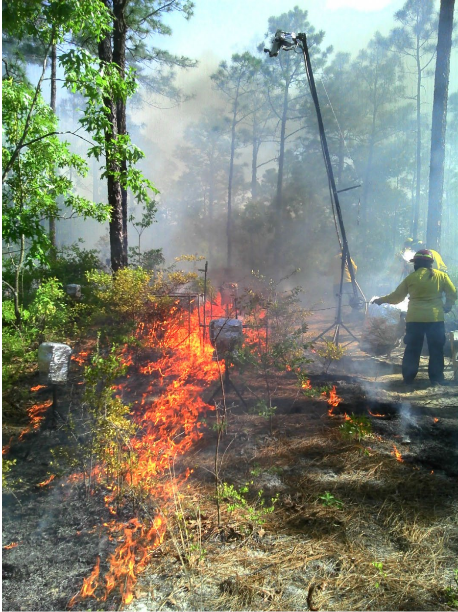
Figure 9 Fire behavior in burn 5 reference plots. A peak total heat flux of 10.9\text{kW/m}^2 was registered for burn 5 along with a peak air temperature of 511^\circ\text{C} , peak horizontal wind speed of 3.8\text{m/s} .
