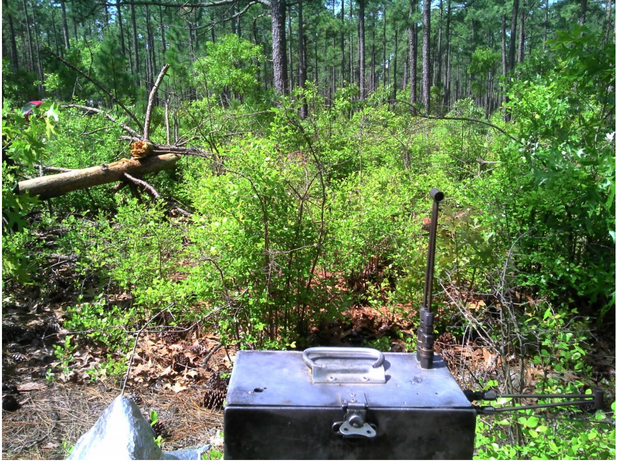
Figure 10 Fuel loading in plot 6. A peak total heat flux of 12.4\text{ kW/m}^2 was registered along with a peak air temperature of 631^\circ\text{C} and peak horizontal wind speeds of 4\text{ m/s} .
