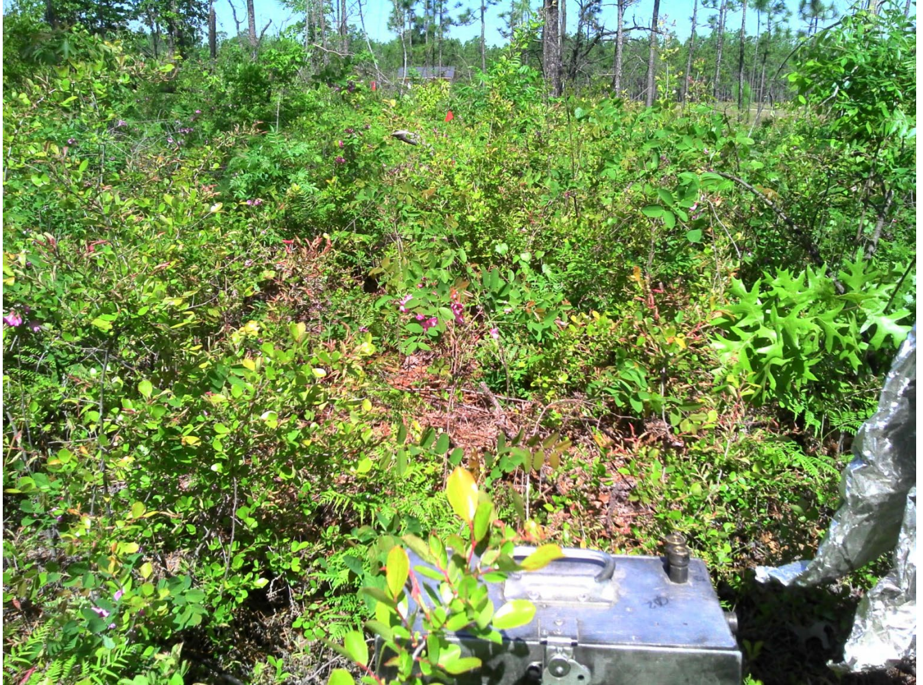
Figure 3 Fuel loading on burn plot 2. A peak total heat flux of 30\text{kW/m}^2 was registered for this burn along with a peak air temperature of 1042^\circ\text{C} and a peak horizontal wind speed of 4\text{m/s} .
